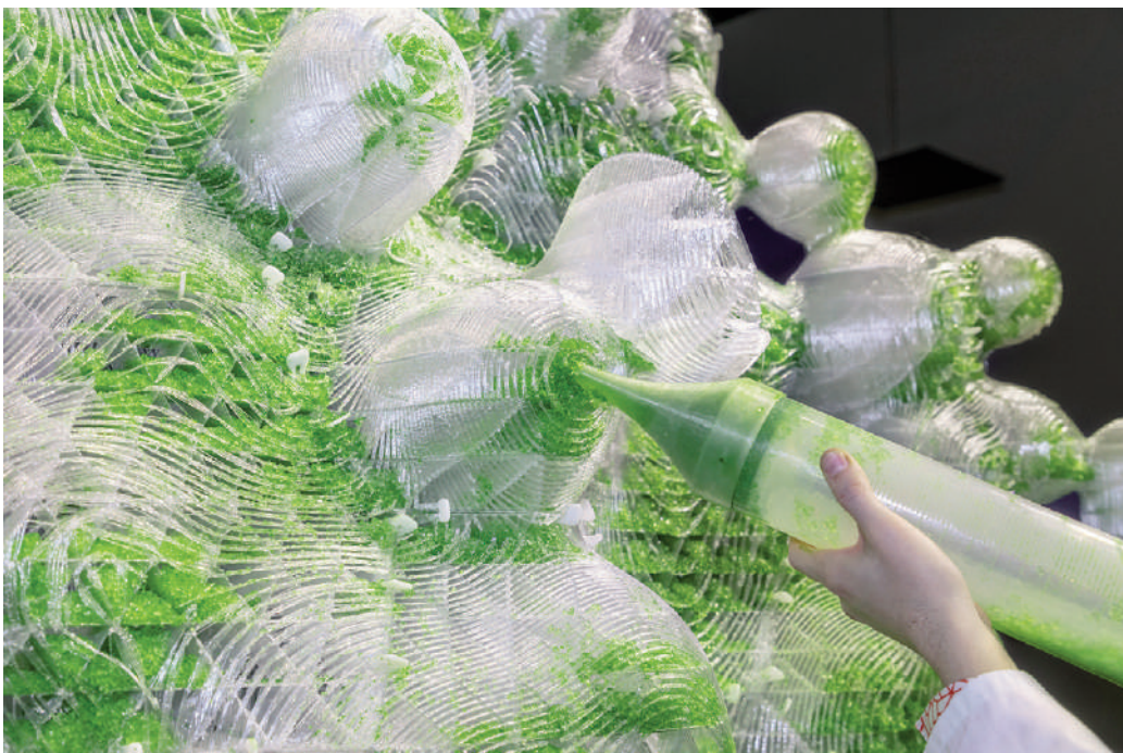
Figg. 11-13 | H.O.R.T.U.S. XL Astaxanthin.g. The world's first 3D-printed bioreactor. The installation, on display at the Centre Pompidou of Paris for the La Fabrique du Vivant exhibit, is understood as a 1:1 prototype of living architecture – a new generation of biophilic architectural skin inserted into urban life. The structure is algorithmically designed and produced through high-resolution, large-scale 3D printing. Among the oldest organisms on Earth, the exclusive biological intelligence of cyanobacteria is collected as part of a new form of bio-digital architecture. Design: ecoLogicStudio (C. Pasquero, M. Poletto, K. Alexopoulos, M. Baldissarra, M. Brewster); Research Partner for biological as well as 3d printed systems and production development: Synthetic Landscape Lab, IOUD, Innsbruck University (Prof. C. Pasquero, M. Kuptsova, T. Greskova, E. Rando, J. Burkart, N. Jabadari, S. Posch), Photosynthetica consortium; Research Partner for 3d printed systems and production development: CREATE Group/WASP Hub Denmark – University of Southern Denmark (Prof. R. Naboni, F. Magaraggia); Engineering: YIP Structural Engineering, M. van de Worp; Microalgal Medium Material Support: Ecoduna AG; 3D printing Material Support: Extrudr (photos by NAARO).
