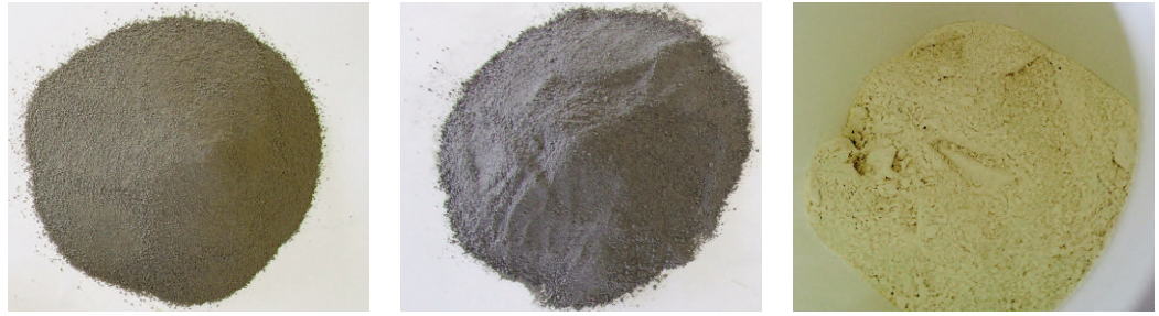
Fig. 12-14 - The materials used in the experimentation: Earth; Sand; Halloysite (credits: Scalisi and Sposito, 2017).
