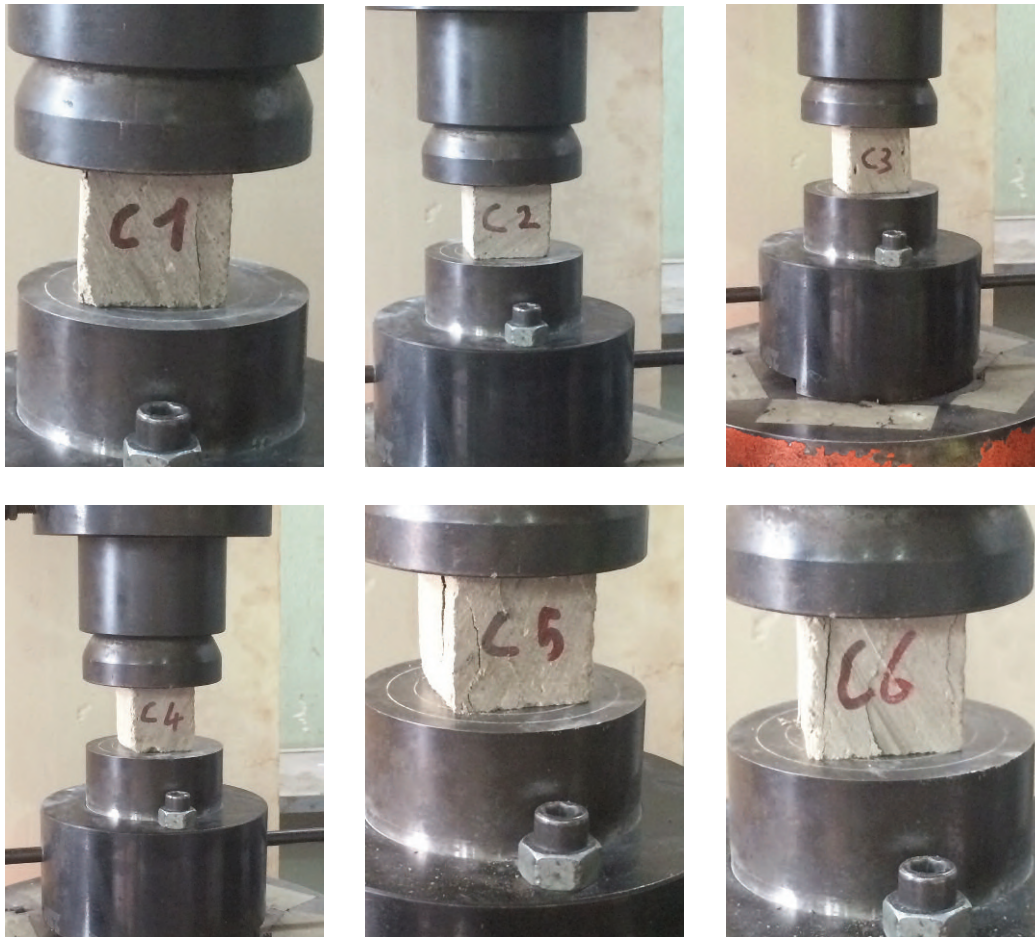
Fig. 21-26 - The samples during compressive strength tests (credits: Scalisi and Sposito, 2017).
