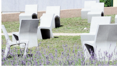
Fig. 8 - Flor, manufactured by Escofet. Playground furniture made of self-compacting reinforced concrete with acid-etched waterproof finishing: colour variation, patina in lower area, staining, and local graffiti (operating life: 4 years); Parco Mennea, Turin (credit: R. Maspoli, 2019).
