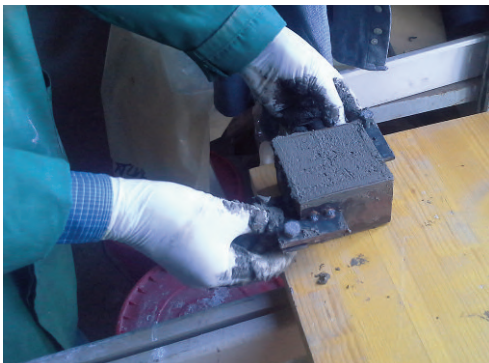
Fig. 15 - Mixture of earth, sand, Halloysite and water (credit: Scalisi and Sposito, 2017).
