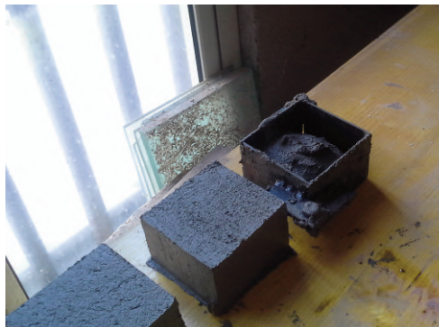
Fig. 15 - Mixture of earth, sand, Halloysite and water (credit: Scalisi and Sposito, 2017).
