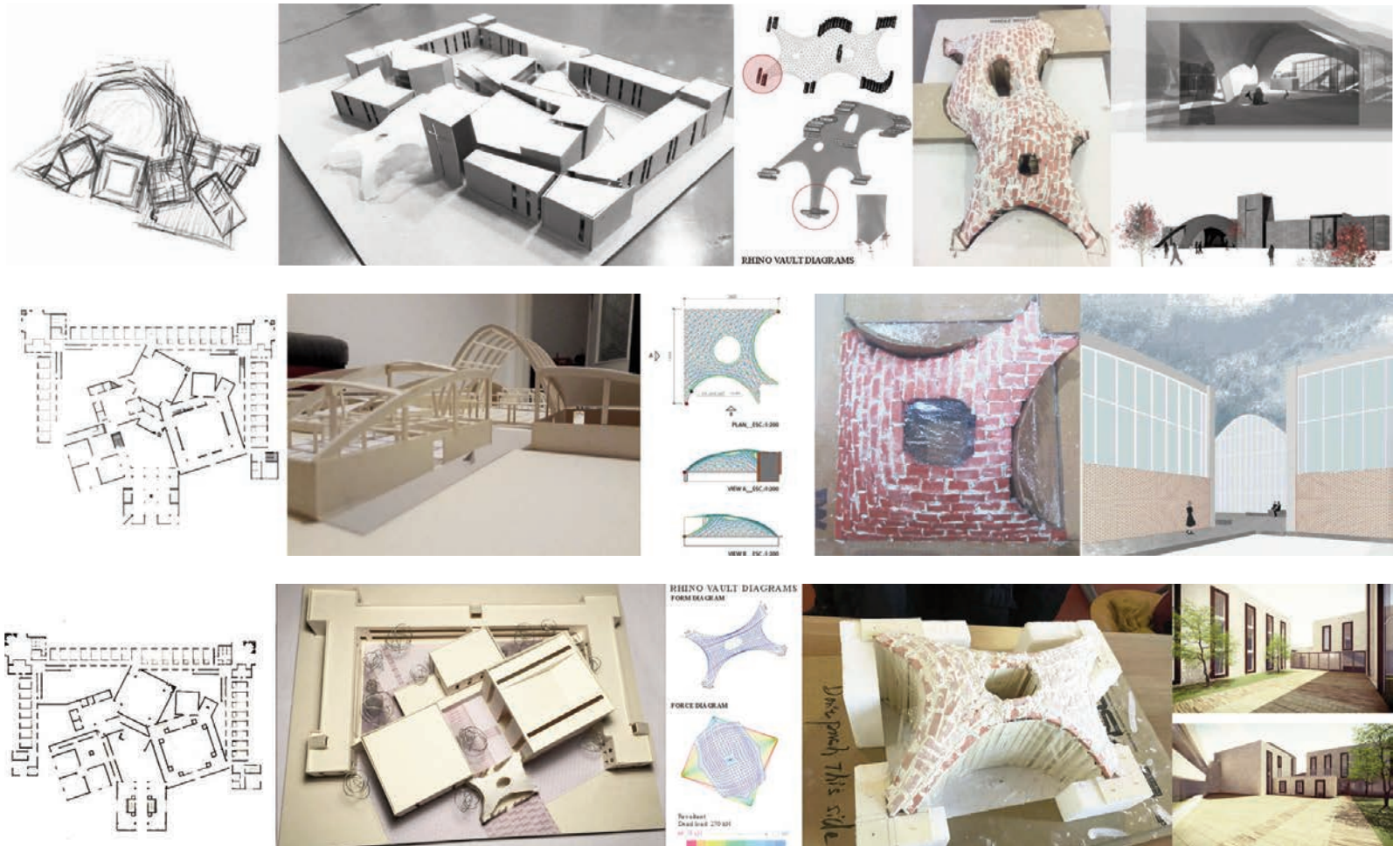
Fig. 1-3 - Work phases in the Design Unit Architecture and Structural Forms: 1) the original project by Louis Kahn; 2) physical model of the students' project proposal; 3) virtual model for verification and remodelling of the project proposal; 4) physical model of the masonry vault as a verification of construction techniques; 5) virtual model of the final architectural proposal (students: M. Di Chiara and V. Attieh; J. Da Costa Real and A. Herrera; H. Liu and G. Piccitto).
