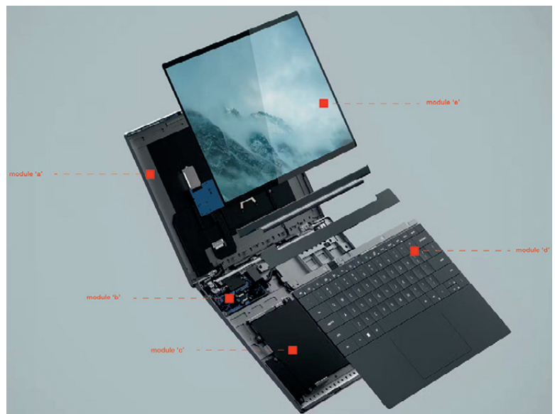
Figg. 12, 13 | Concept Luna prototype: 13" notebook designed with a series of modules that can be easily disassembled and connected via interlocking and reversible connections; the main modules ('a'+ 'b'+ 'c'+ 'd'+ 'e') that configure the notebook (credits: Dell Inc.).
