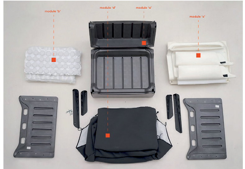
Figg. 7, 8 | Costume Armchair and main modules of the Armchair version: the armchair core 'a'; the seat, composed of a spring insert 'b' and a polyurethane layer 'c'; the fabric cover 'd' (credit: Magis).
