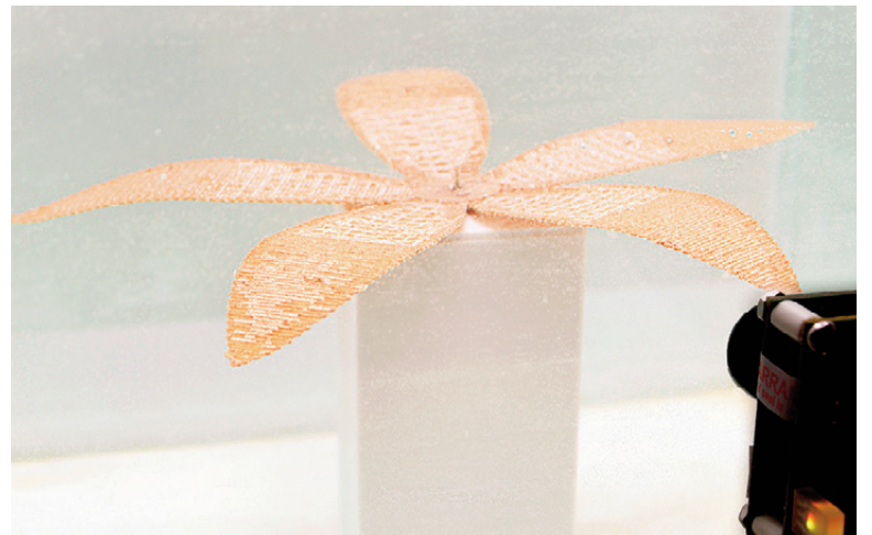
Fig. 10 | Top view of the actuator before being exposed to humidity (0 minutes) and after 60 minutes of immersion (credit: G. Pelliccia, 2023). Fig. 11 | A fixed camera was positioned in front of the glass box to acquire one photo per minute (credit: G. Pelliccia, 2023).
