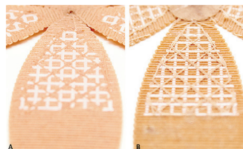
Fig. 4 | Different raster patterns were used for the various functional modules: the zig-zag RP optimizes the expansion of Laywood orthogonally to the print direction, the grid 90° RP ensures an effective constraint to the hygro-expansion of Laywood, and the grid 45° allows to bond together Laywood and PLA through multiple contact points (credit: G. Pelliccia, 2023).
