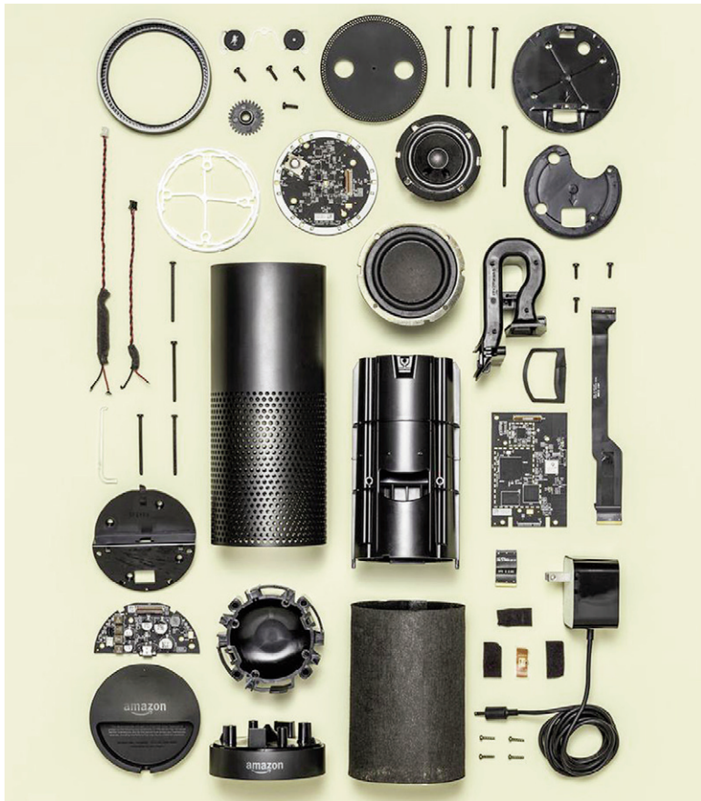
Fig. 11 | Physical components of 'Alexa', Amazon Echo (credit: T. McLellan, 2017).
