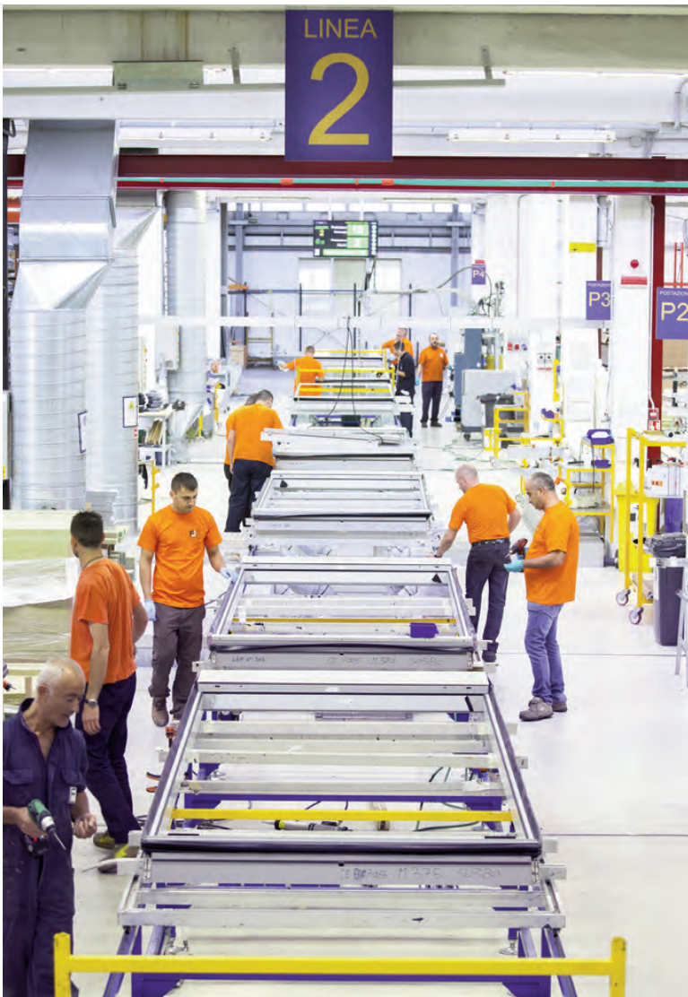
Fig. 1 | In-line production of curtain wall modules (credit: G. Salvatori, 2015).
