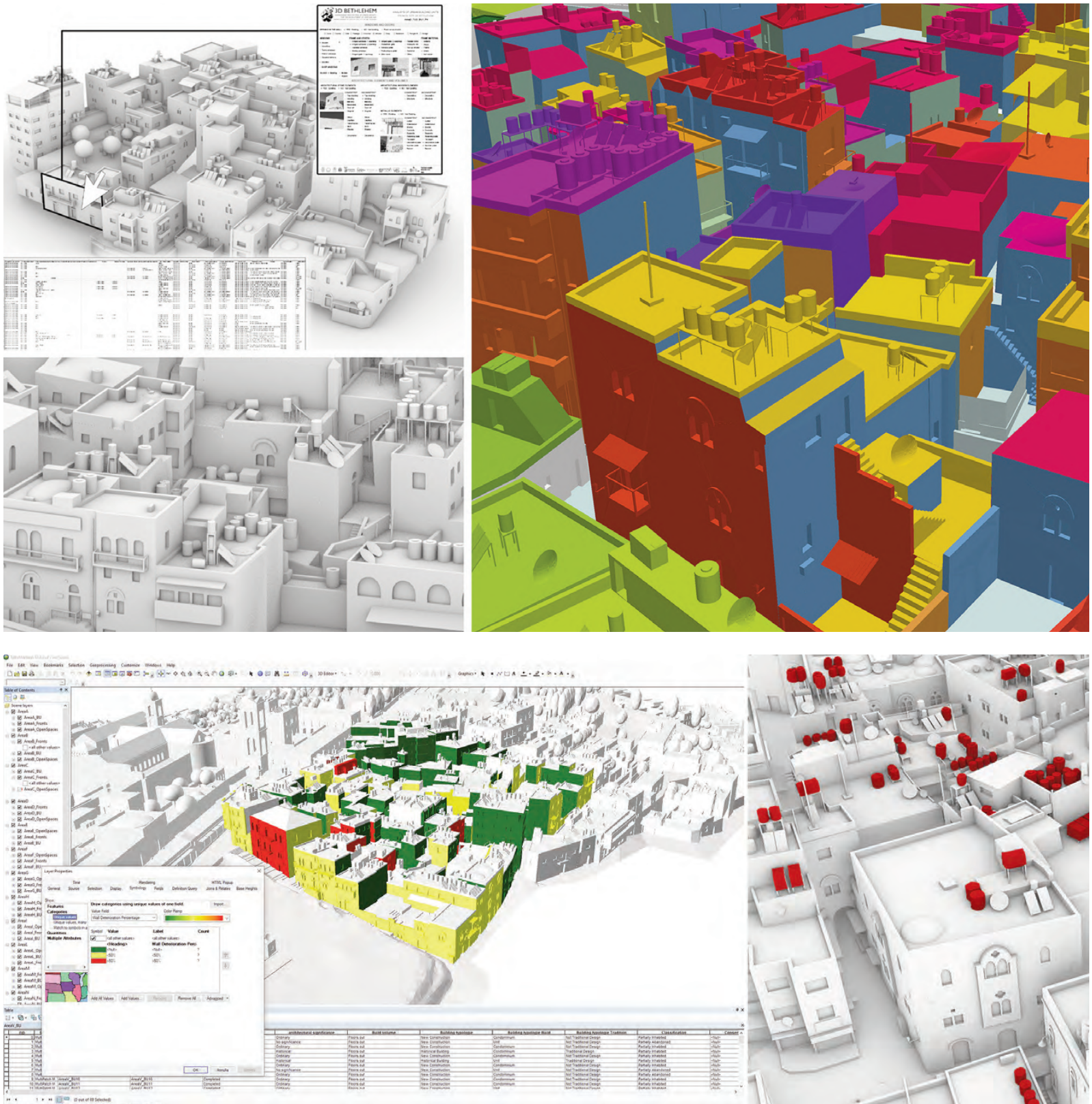
Fig. 13 | Three-dimensional model created during the 3D Bethlehem project: on the left, the model imported into the GIS environment with sample diagram of the urban census connections to the platform; on the right, an image of the application of thematic maps to the model, which are derived from the visualization of census data (credit: E. Doria, 2022).
