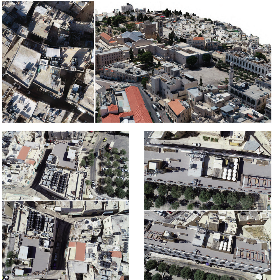
Fig. 5 | On the left, an orthoimage obtained by processing a three-dimensional mesh model from a photogrammetric point cloud from UAV; on the right, a portion of the textured model generated from photogrammetric acquisitions of Bethlehem's historic center (credit: E. Doria, 2022).
