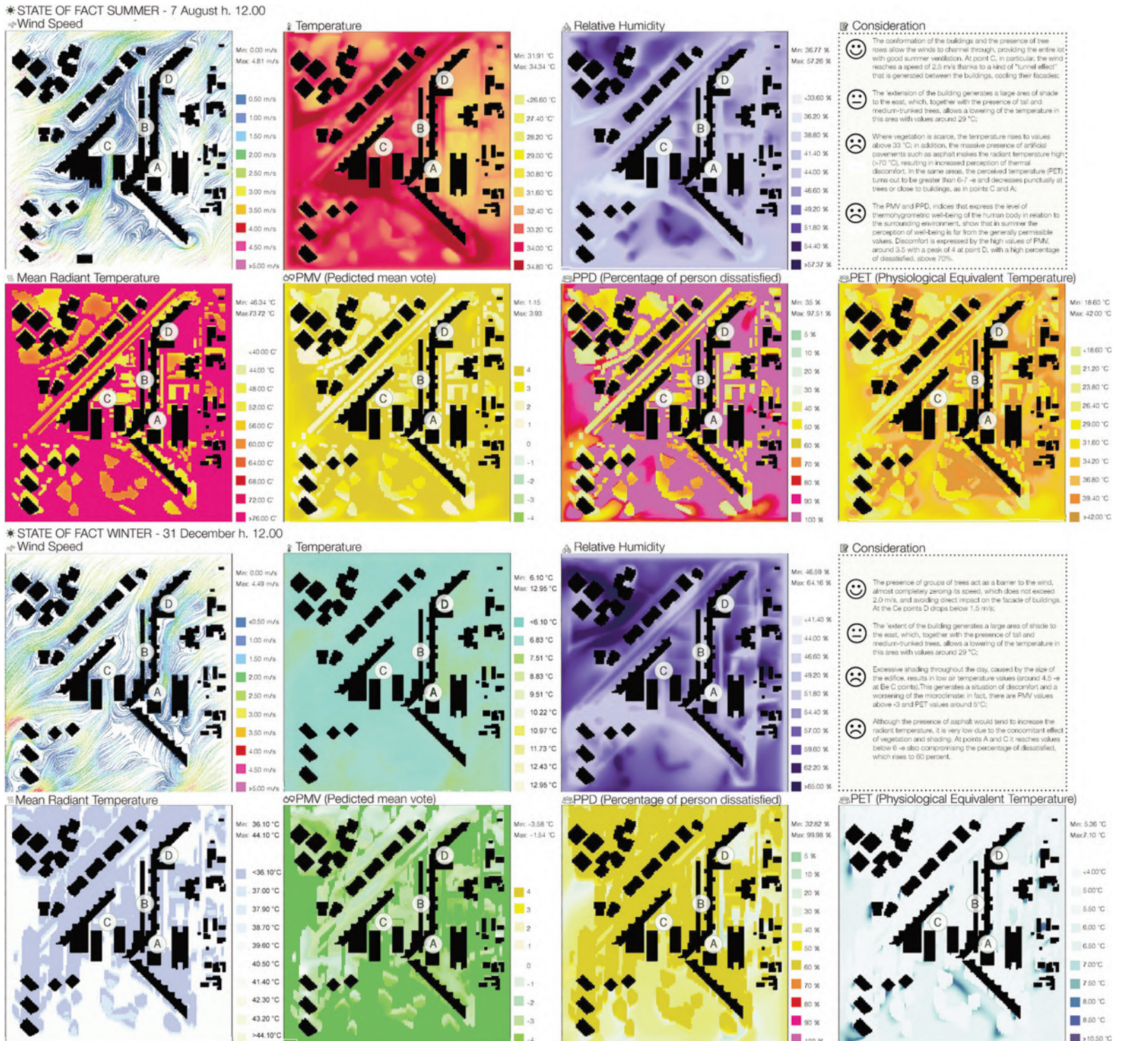
Fig. 6 | Ante operam fluid dynamics simulations of the Vigne Nuove 'Piano di Zona', Rome (credit: the Authors and C. Dalsasso, 2021-2022).
