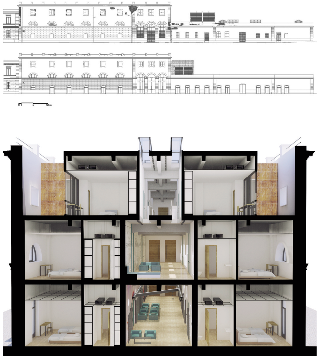
Fig. 7, 8 - From the top: Overview of the present state and of the project on via Beniamino Franklin; Perspective section of the three-storey volume.
