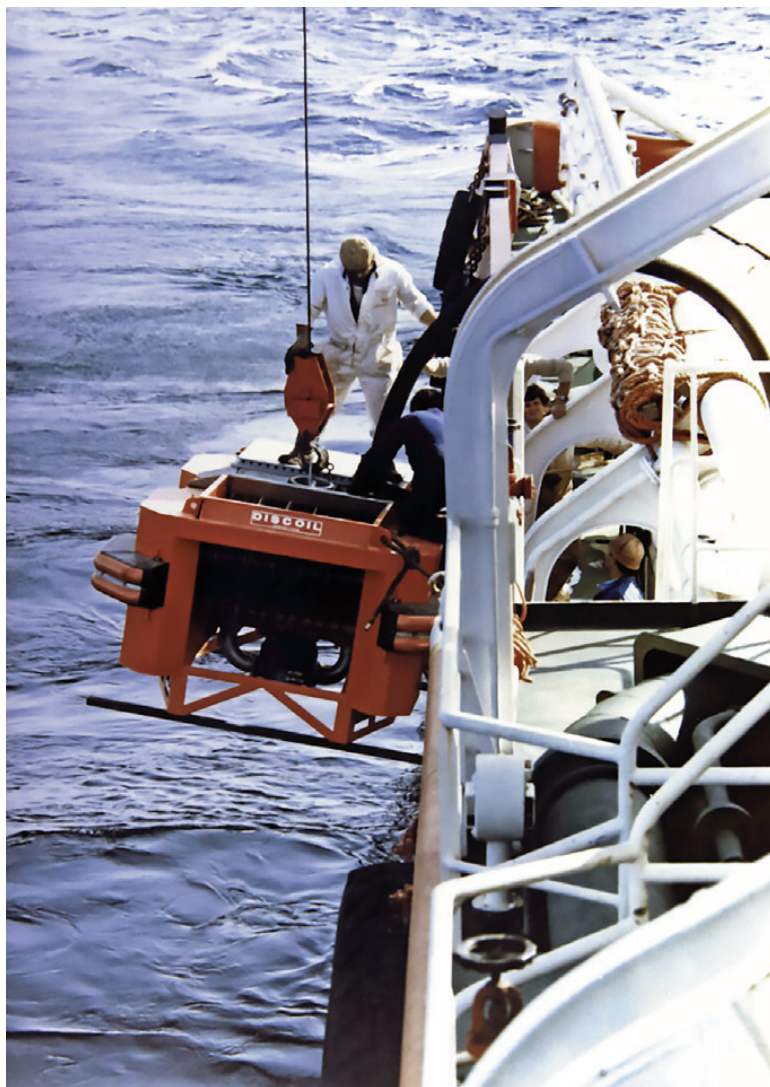
Fig. 6 | The configuration of the Floating Discoil dedicated to spill pollution (credit: OCS, 2006).
