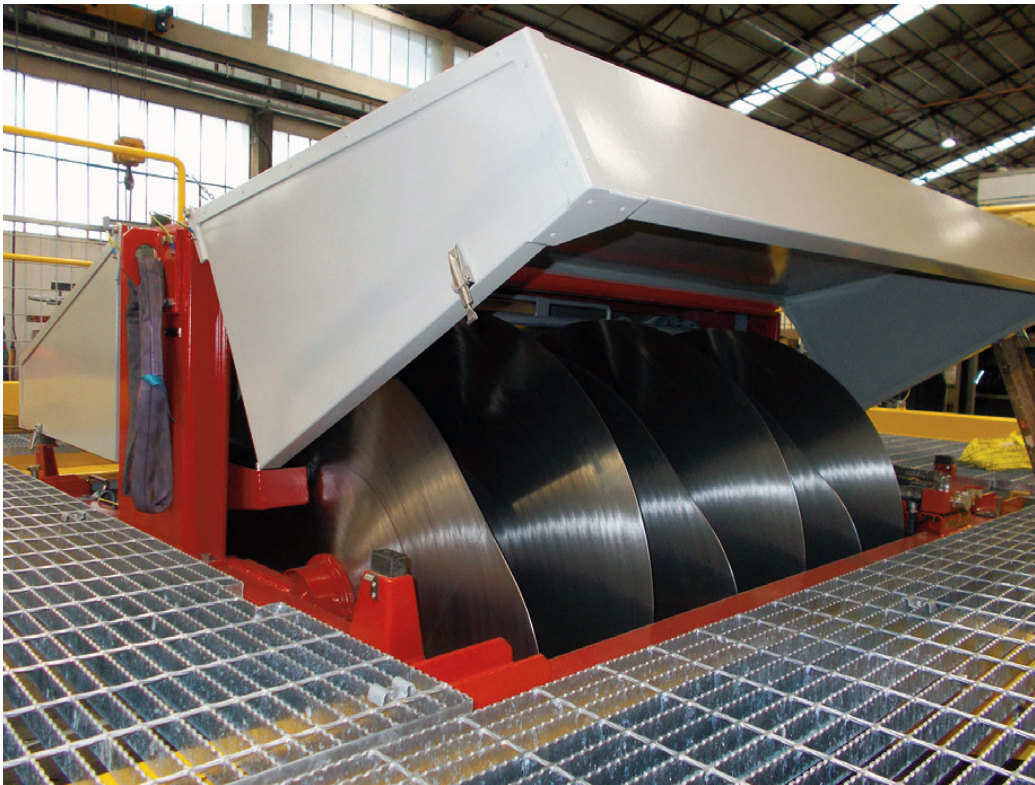
Fig. 2 | The disc structure of the current Discoil oil separator (credit: E. Marchetto, 2018).
