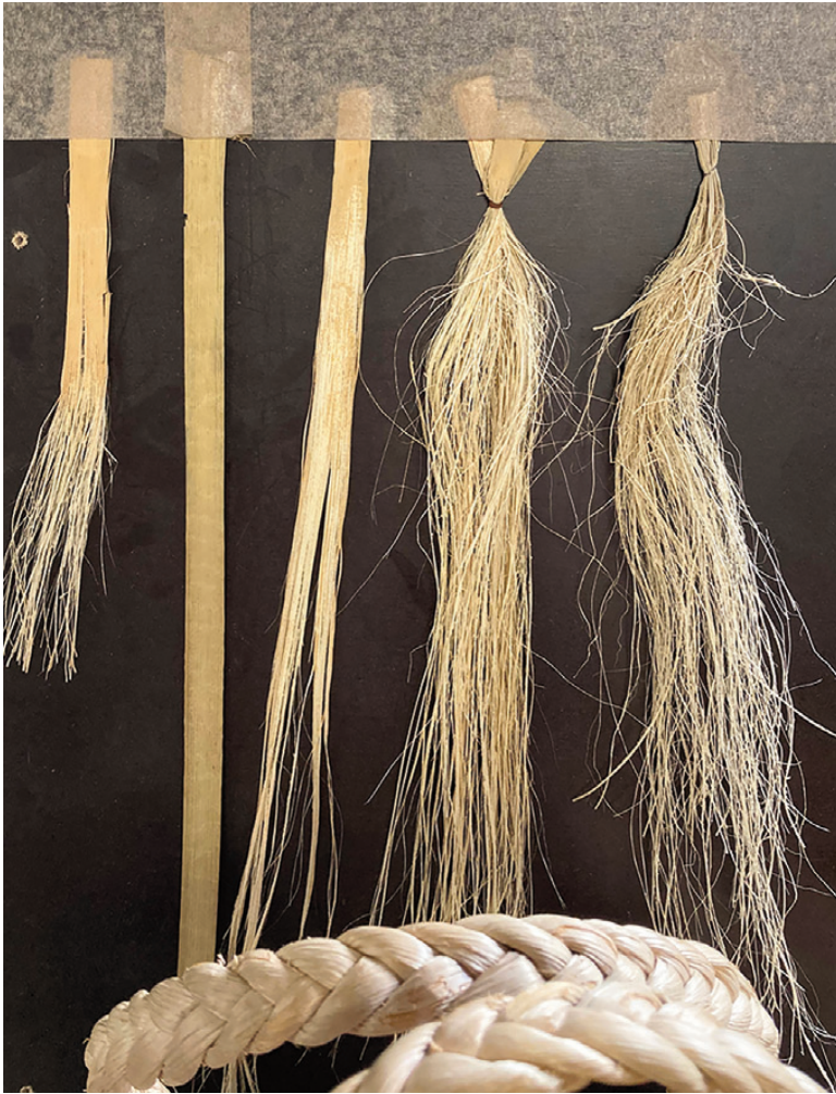
Fig. 8 | Typha fibres extraction samples made by RietGoed (credit: E. Morpurgo, 2024).
