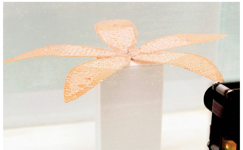
Fig. 10 | Top view of the actuator before being exposed to humidity (0 minutes) and after 60 minutes of immersion (credit: G. Pelliccia, 2023).
