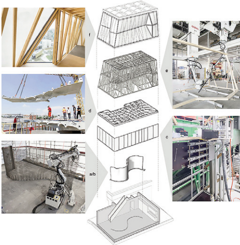
Fig. 6 | Main features of the 4D printing process (credit: the Authors, 2023).
