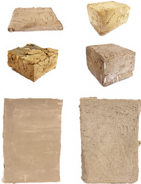
Fig. 8 | Experiment: Foam soaked in clay and covered with different thicknesses and densities (credit: IAK, S. Jaza, M. Schulze Gronover).
