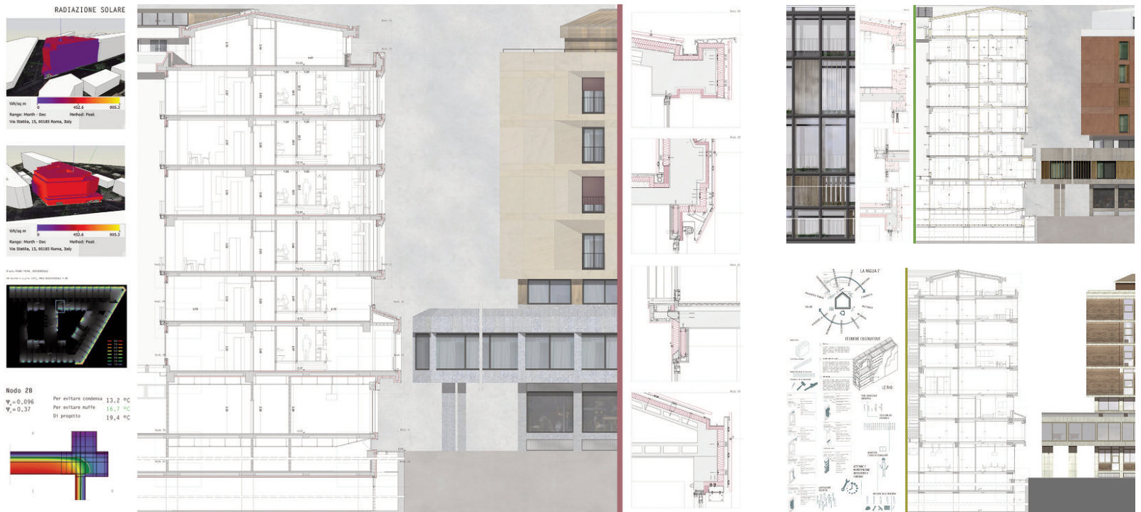
Fig. 16-18 - Example images of the three energy analysis and retrofit scenarios carried out through solar analysis, lighting control, hygrothermal analysis, technological details of envelope. The three scenarios represented, in order are: sustainability scenario, efficiency scenario, self-help scenario (drawings by S. D'Arcangeli, M. Gesmini and I. Grossi, 2017).
