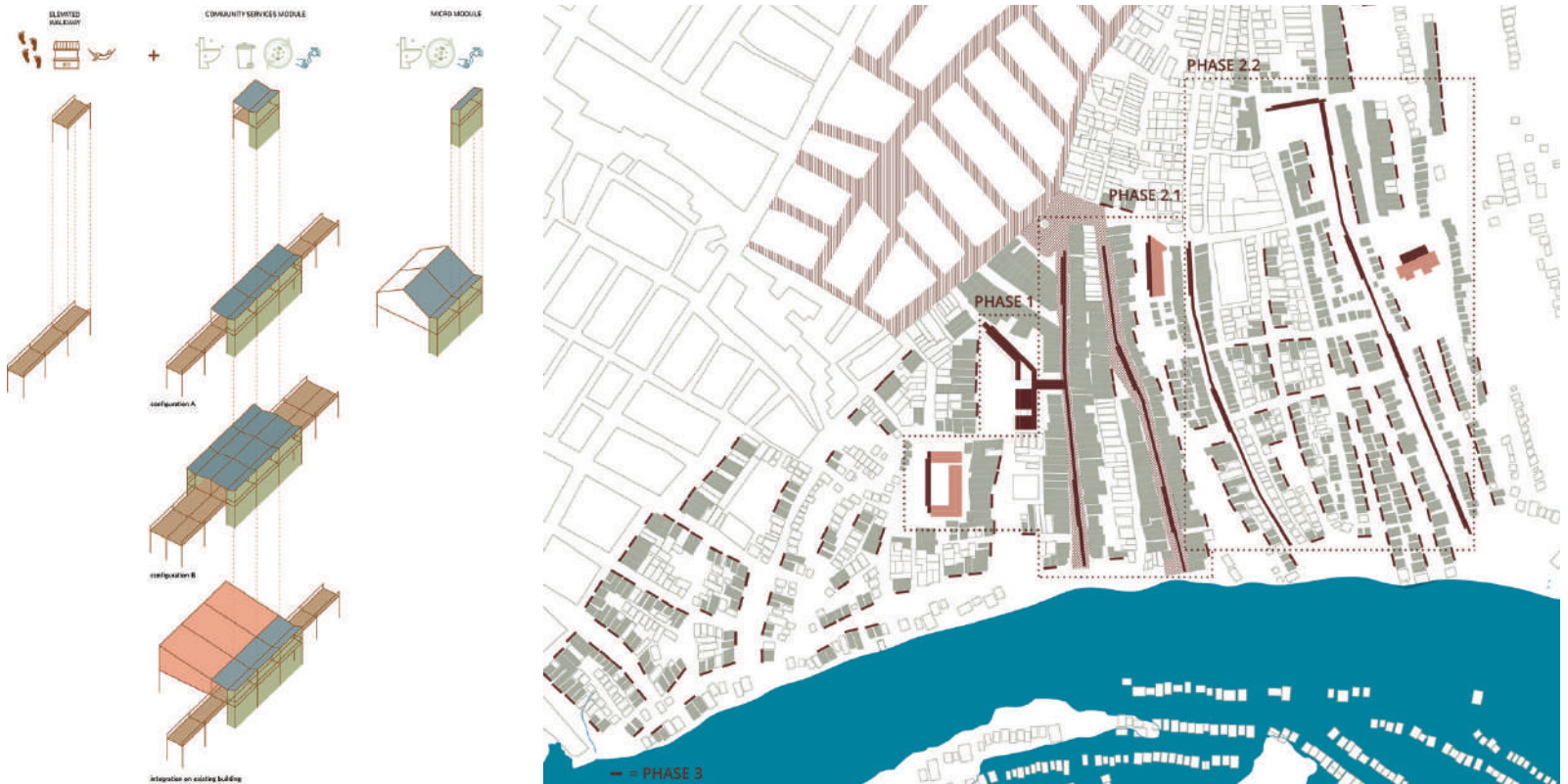
Figg. 8, 9 | Operation scheme of the modules; Layout of the intervention in the lower area of Belén.
