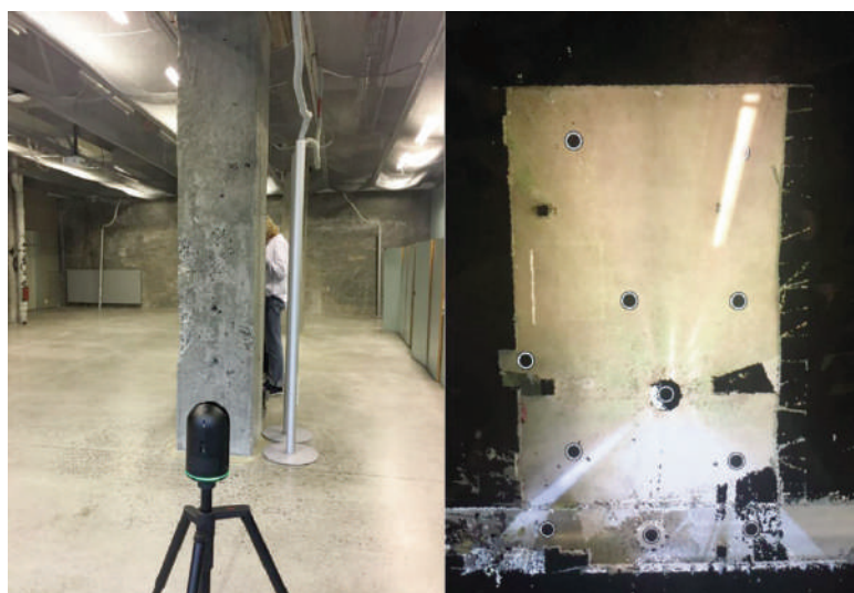
Fig. 3 | Typical 3d scanning scenario: Leica BLK360 Scanner; Interface on Ipad Pro (credit: K. Reaver, 2018).
