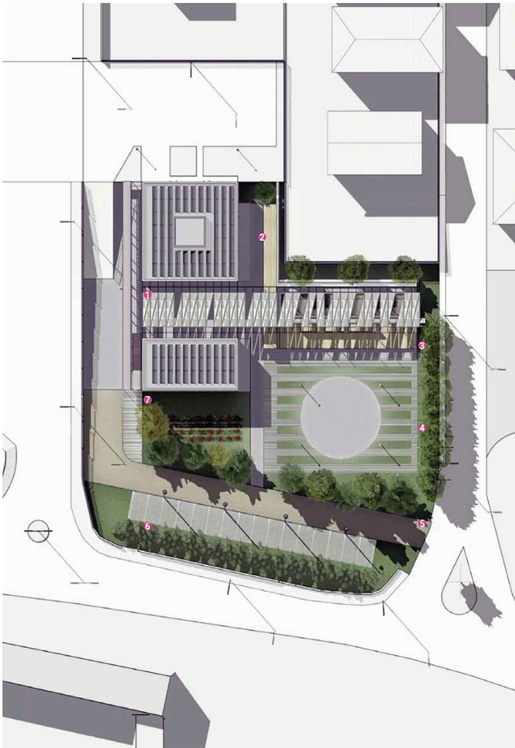
Fig. 12 | Project for the Lighthouse 7 in Nepi, General Plan (2024): 1) solar tents; 2) social public laundry; 3) furnished stage for public events and continuous seating; 4) new public square with porous soil; 5) tree-based acoustic filter towards the road; 6) parking set up as rain garden and phytoremediation area; 7) urban horticulture. The project is designed by Rimond in collaboration with the Architectural Department of Roma Tre University (credit: Rimond, 2024)
