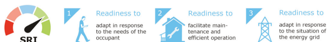
Fig. 2 | Three key functionalities of smart readiness in buildings (source: European Commission et alii, 2020).
