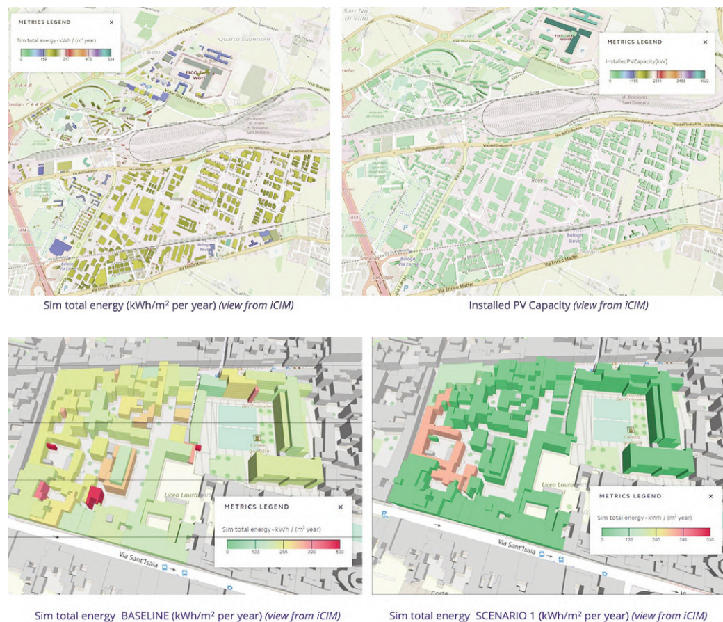
Fig. 7 | Pilastro / Roveri district, Bologna: Simulation model of the district's energy consumption; Simulation of the potential for electricity production from the installation of photovoltaic panels (source: projectgreta.eu; r2msolution.com).
