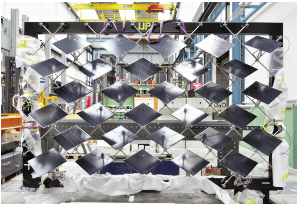
Fig. 2 - Arno Schlüter, Adaptive solar façade prototype including soft robotic actuators (credit: www.ita.arch.ethz.ch/chairs/architecture-and-building-systems.html ).
