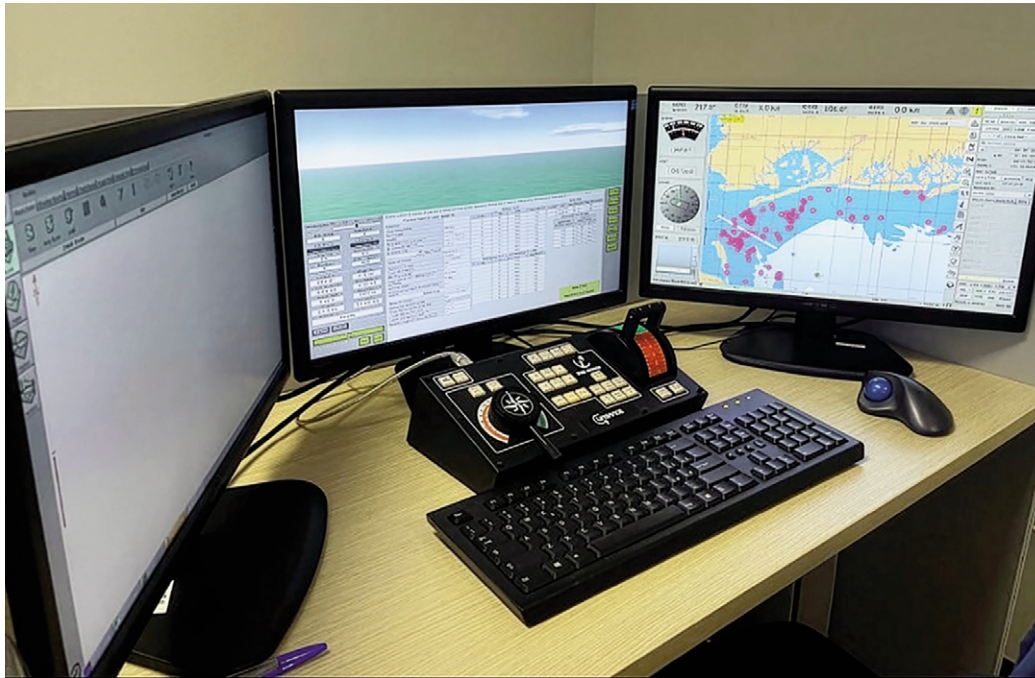
Fig. 5 | Full mission bridge simulator used in the cooperative scenario for analysing coordination dynamics and team cognitive workload (credit: the Authors, 2026).
