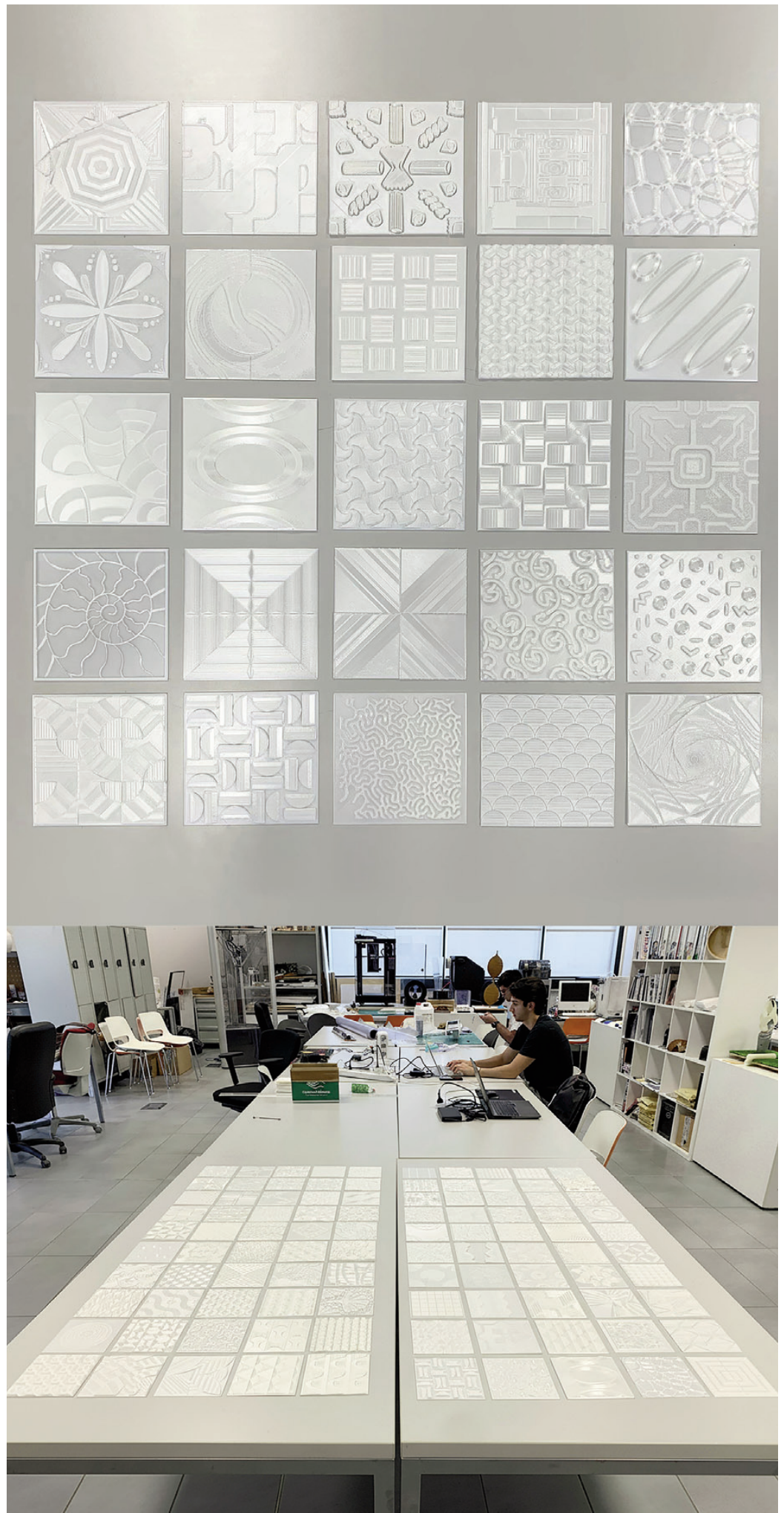
Fig. 15 | Samples for the study tests carried out in the laboratory by means of rapid prototyping Fused Deposition Modelling in PLA (credit: the Authors, 2026).
