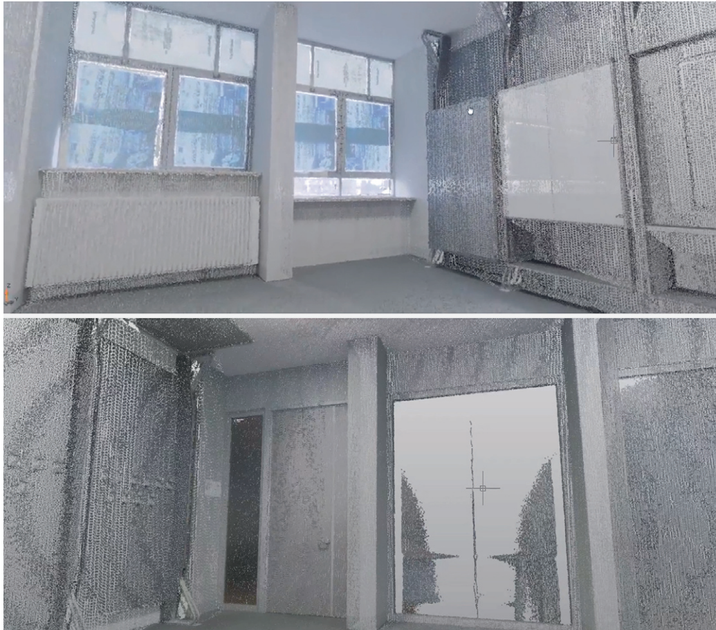
Fig. 7 | Processing of the point cloud acquired by the Leica BLK360 G1 laser scanner: two screenshots of the Leica Cyclone Register 360 software used to process data from the survey of the sample classroom at the 'Fermi Sacconi Ceci' ITT (credit: the Authors, 2025).
