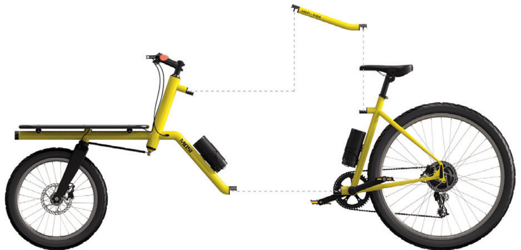
Fig. 8 | E-cargo bike layout, Size 'M': modules and disassembly scheme (credit: the Authors, 2025).
