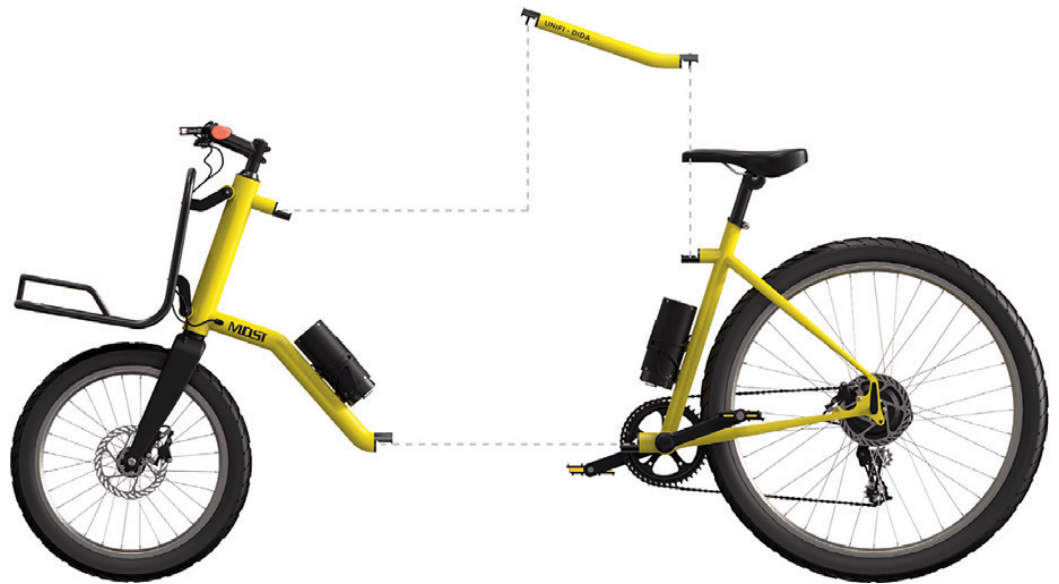
Fig. 7 | E-cargo bike layout, Size 'S': modules and disassembly scheme (credit: the Authors, 2025).
