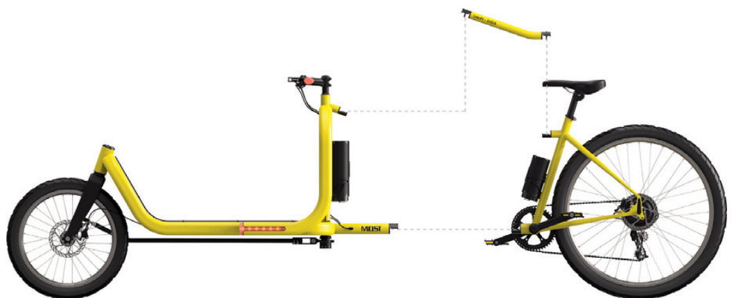
Fig. 9 | E-cargo bike layout, Size 'L': modules and disassembly scheme (credit: the Authors, 2025).
