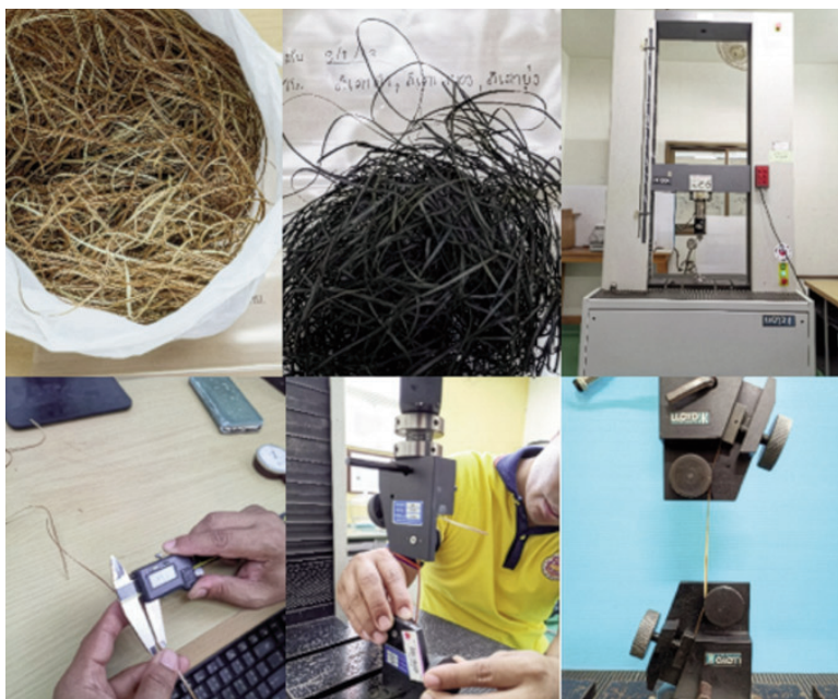
Fig. 7 | Mechanical testing procedure used to analyse the structural behaviour and flexibility of 'yanlipao' fibres (credit: the Author, 2020).
