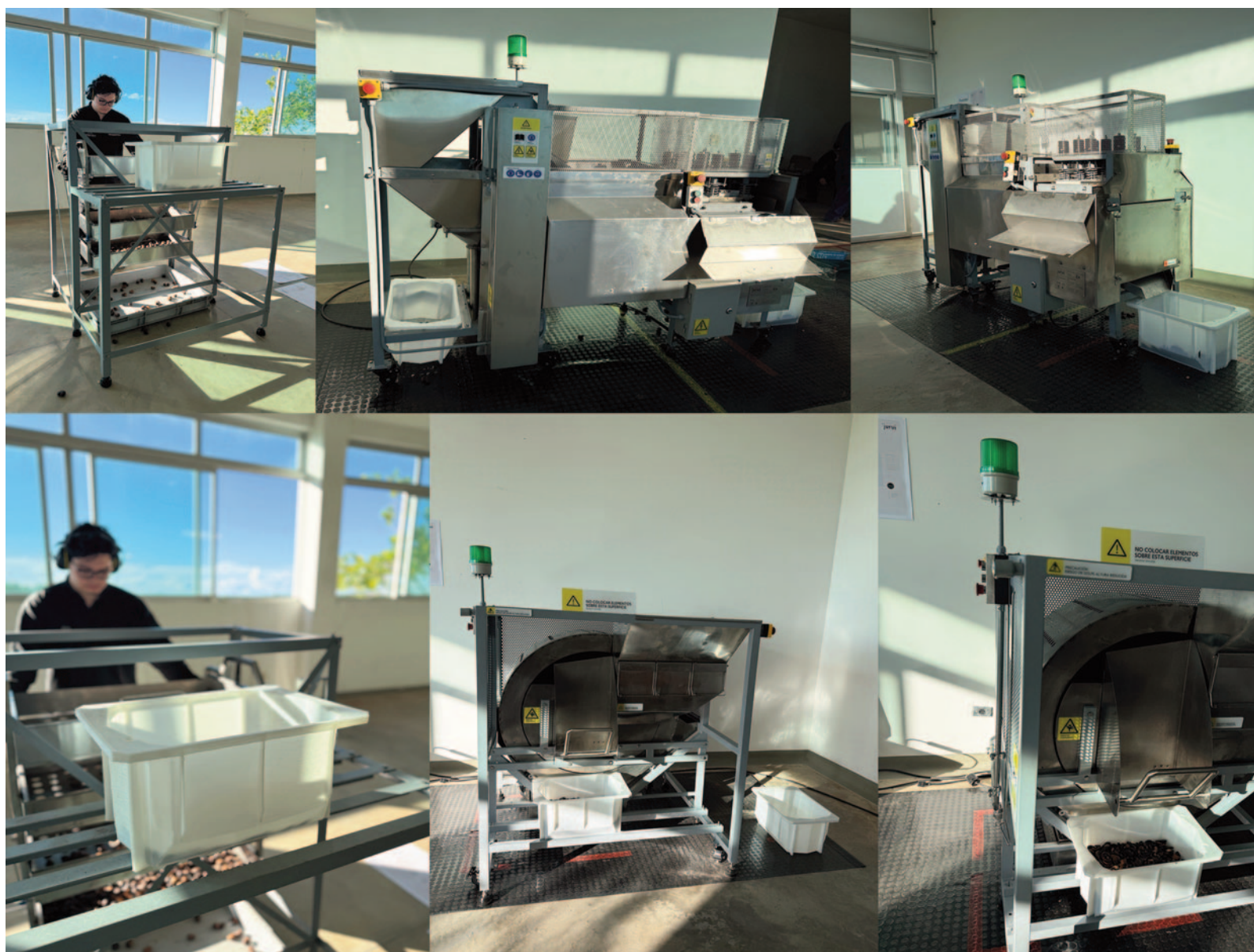
Fig. 13 | Compatibility testing of the redesigned basket with R&D prototypes for cashew nut opening, separation, and classification in Vichada (credit: Jurui Project, 2024).
