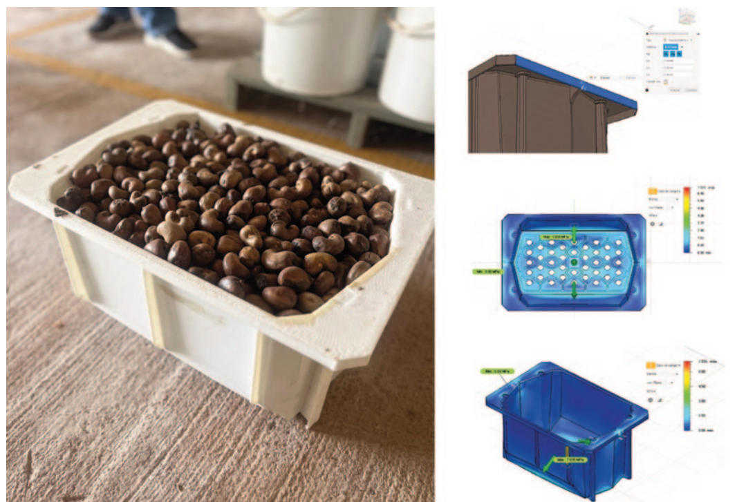
Fig. 19 | Field validation assessing transfer efficiency, spillage during pouring, and stacking stability during transport (credit: Jurui Project, 2025).
