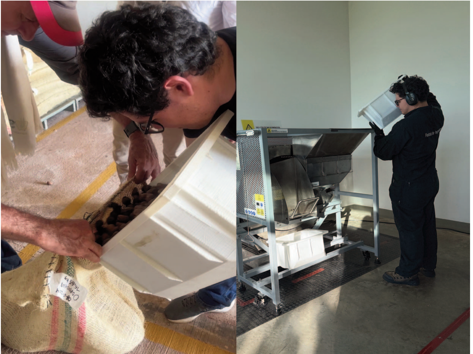
Fig. 14 | Controlled pouring tests using sacks and prototype receivers to evaluate rim geometry and wall inclination to reduce spillage (credit: Jurui Project, 2025).
