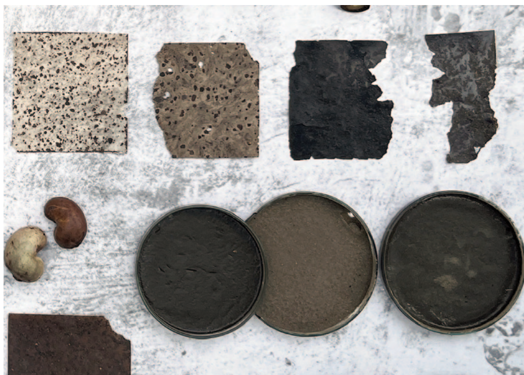
Fig. 7 | Laboratory experiments combining cashew shell residues with biodegradable polymers to develop composite materials (credit: Jurui Project, 2023).
