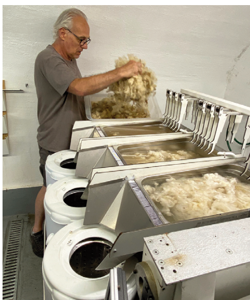
Fig. 11 | Case study of a scouring machine designed by the 'Pro Verzasca' association (credit: Design Friction Lab, 2025).
