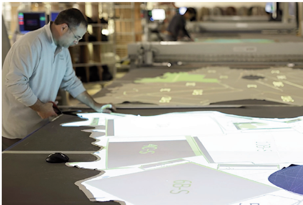
Fig. 5 | Digital optimisation of nesting during the cutting phase of upholstery semi-finished components, aimed at improving material efficiency and reducing production waste in sofa manufacturing (credit: Natuzzi Group, 2026).
