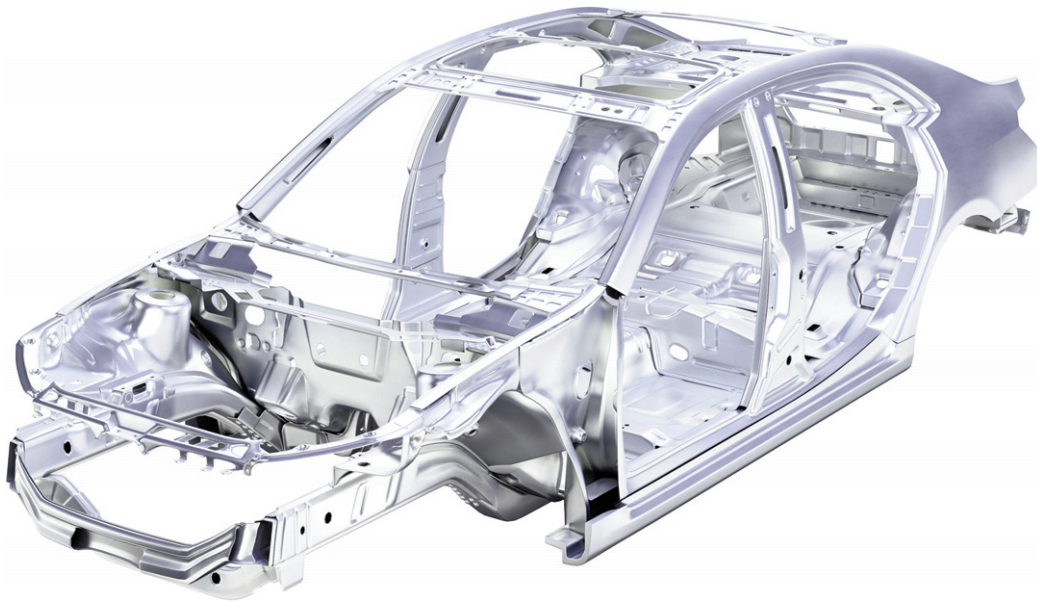
Fig. 1 | BIW design and monocoque structure (credit: Kutz, 2011).
