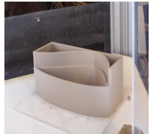
Fig. 6 | From digital model to prototyping: parametric modelling phase and additive production of a sub-component of The Dome Wall system through the Liquid Deposition Modelling process (credit: the Authors, 2026).
