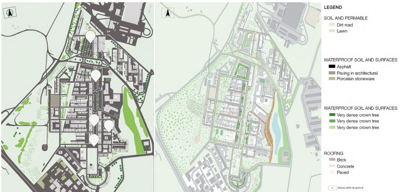
Fig. 10 | Mapping of the materials and the outdoor spaces ante and post operam of the Casal Monastero 'Piano di Zona', Rome (credit: the Authors and S. Urbinati, 2021-2022).
