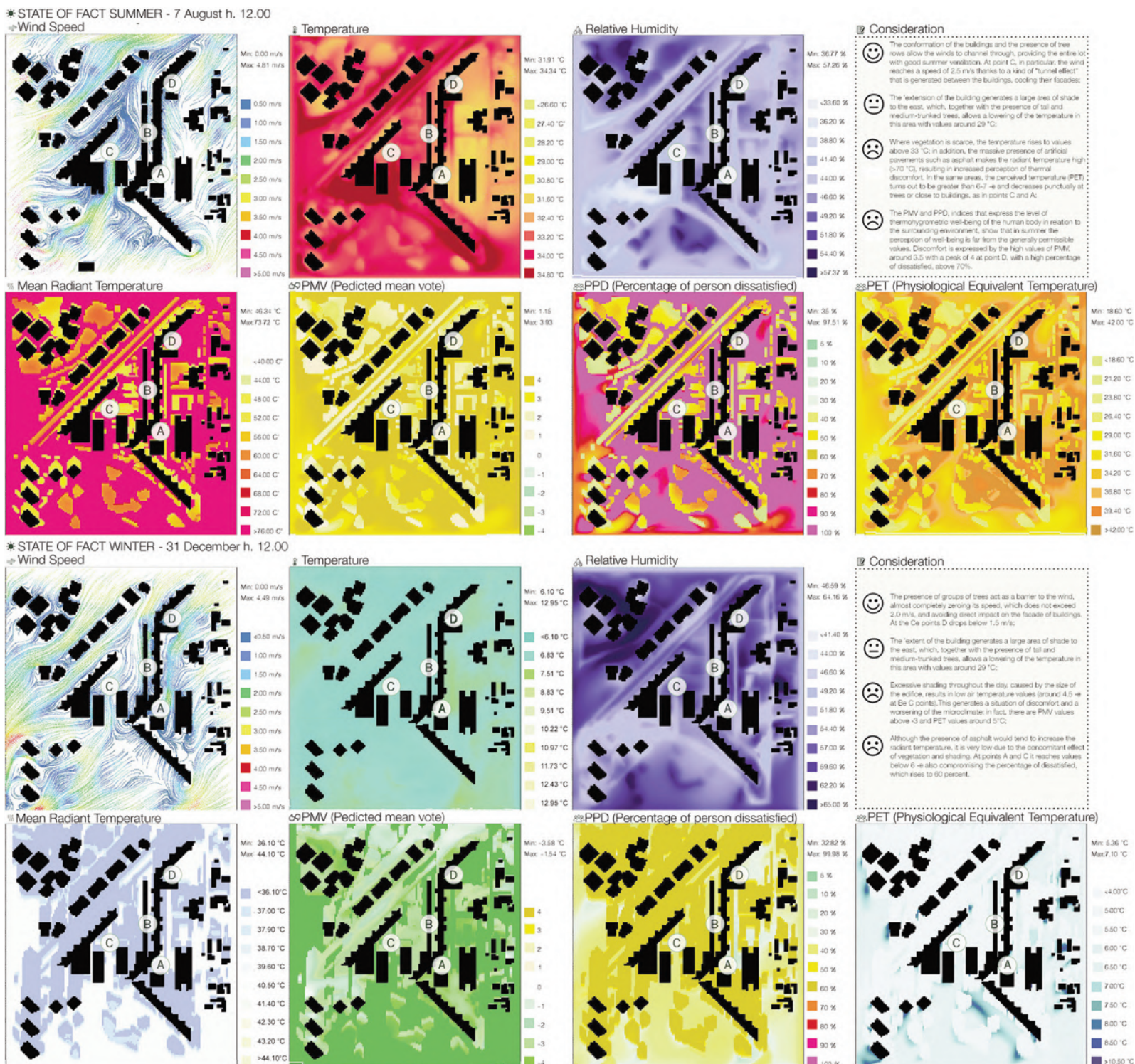
Fig. 6 | Ante operam fluid dynamics simulations of the Vigne Nuove 'Piano di Zona', Rome (credit: the Authors and C. Dalsasso, 2021-2022).
